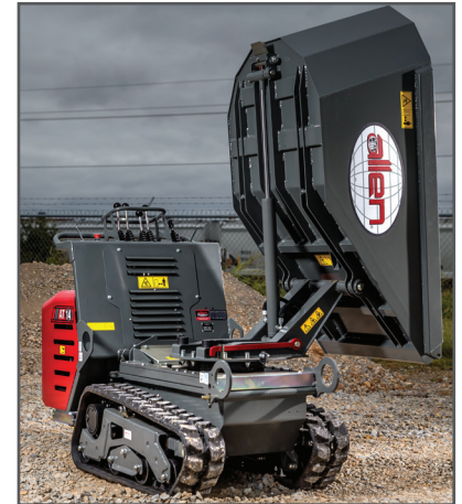
Swivel design allows bucket to turn 90° in either direction from center.
